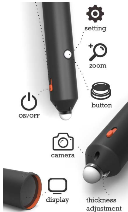
Figure 1. Design elements on the stylus of Colode
